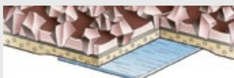
Butted joint with special film on the back
