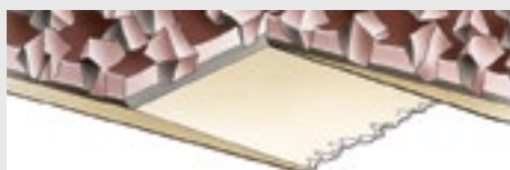
Overlapped joint without grit sanding
