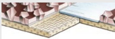
Butted joint with special film on the grit side
