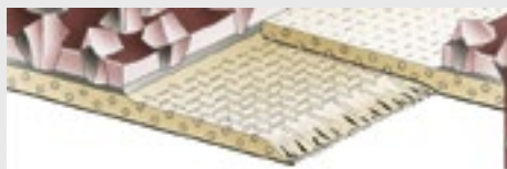
Overlapped joint with grit sanding
